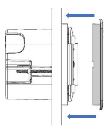
3. Make sure the four dedicated locking tabs snap correctly into place to ensure proper attachment and operation.
