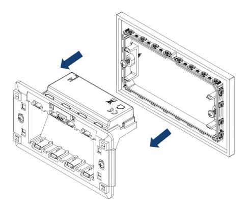
**IMPORTANT:** Make sure the power breaker / fuse is flipped and no hazardous voltages are present at the installation point before proceeding.
