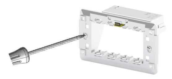
**NOTE:** When *Smart Diffuser* is present, use 3.5x22mm screws that come with the *Diffuser*. When no *Diffuser* is present, use 3.5x16mm screws that come with the *Smart Frame*.
