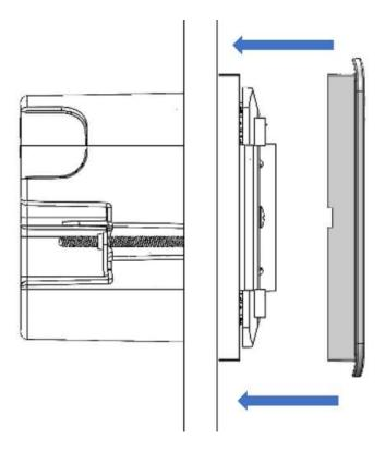
3. Make sure the four dedicated locking tabs snap correctly into place to ensure proper attachment and operation.
