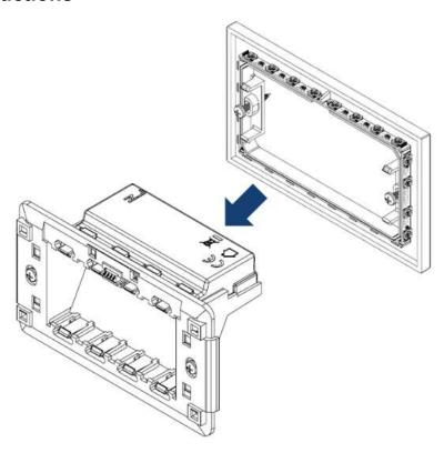
1. Before the following steps, asure the orientation of the *Connekt Smart Diffuser 4M* matches the orientation of the *Connekt Smart Frame 4M*. The connector on the *Diffuser* should match the position of the connector on the Frame, both facing upwards.
