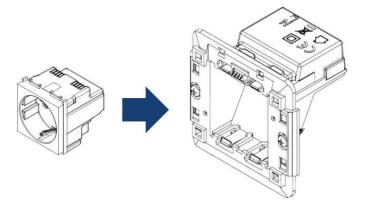
1. Attach selected modules to the *Connekt Smart Frame*. The user can select any compatible modules from *Connekt Smart* and *Connekt Regular* series of products according to personal requirements and preferences.
