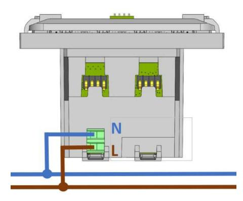
**IMPORTANT:** Make sure the wires are adequately inserted and terminal screws are properly tightened.
