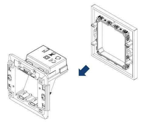
1. Before the following steps, asure the orientation of the *Connekt Smart Diffuser 2M* matches the orientation of the *Connekt Smart Frame 2M*. The connector on the *Diffuser* should match the position of the connector on the Frame, both facing upwards.
